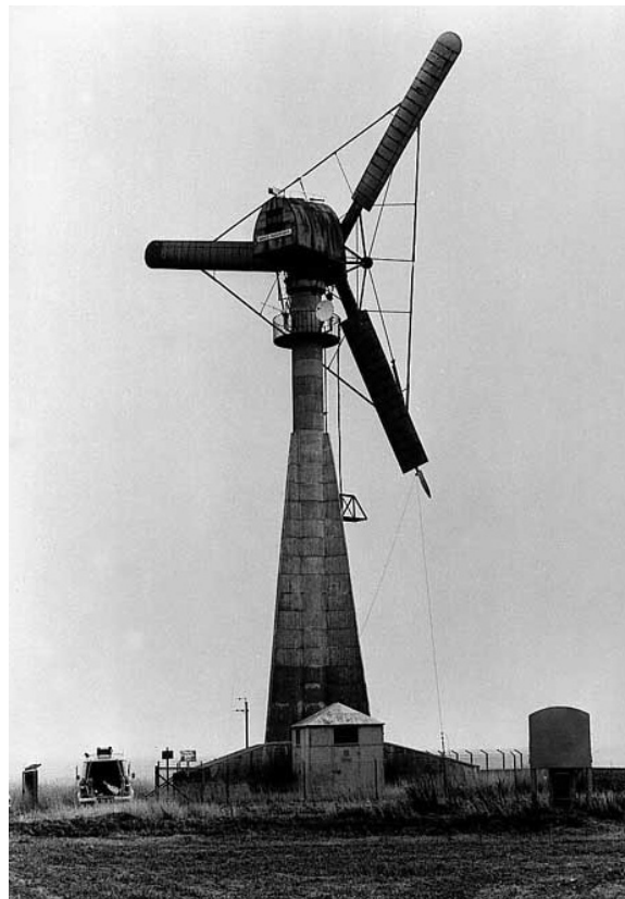
Figure 13. Emergency rotor tip brakes for the Gedser stall controlled wind turbine. Source: Danish Wind Turbine Manufacturers Association.
