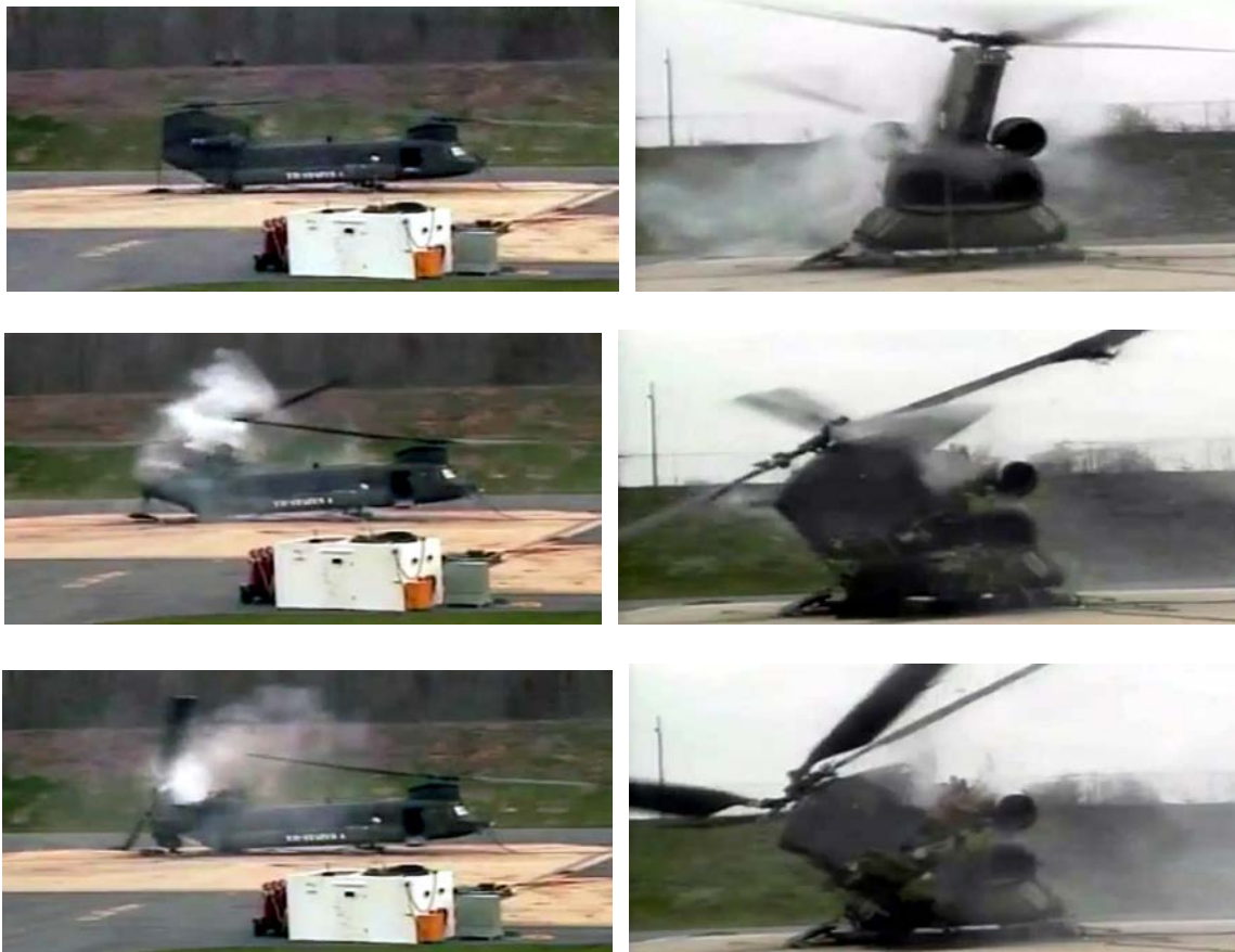
Figure 9. Resonance failure testing of helicopter blades.
