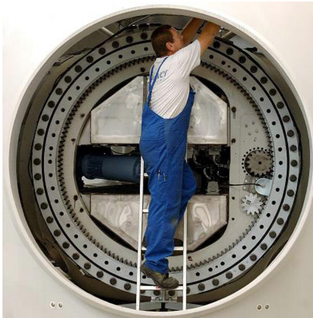
Figure 24. The gear boxes of wind turbines need replacement every five years, as they are the component that is most prone to failure from wind gusts causing misalignment of the drive train. Source: Der Spiegel, DPA.
