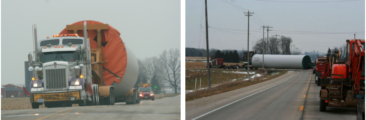
Figure 25. Difficulty in moving turbine components on existing rural roads.
