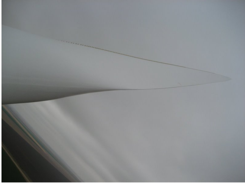
Figure 22. Structural crack caused by manufacturing defect in a rotor blade.
